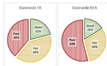
Figure 14 (A) Left: Statewide paved county primary road network conditions by percentage of good, fair, or poor. Right: Statewide unpaved county primary road network conditions by percentage of good, fair, or poor.
