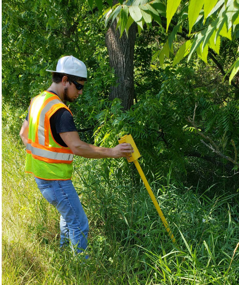
Figure 6-2: Oceana CRC using a metal detector to try and locate a culvert
