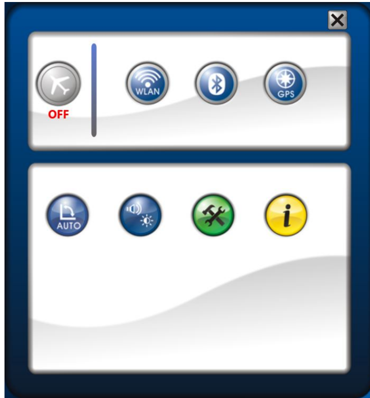
Figure 14 - Quickmenu Control Screen – if the GPS icon in the upper-right is blue the GPS is running
