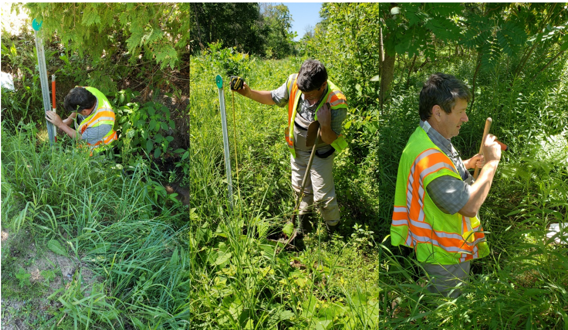
Figure 7-6: A graduated rod, tape measure, and sight level were also used to determine depth of cover
