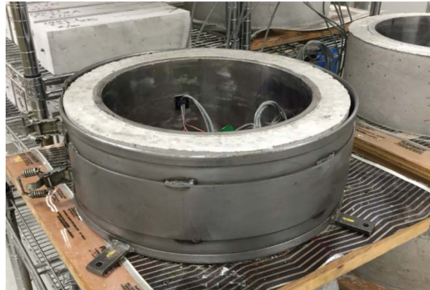
Restrained shrinkage crack ring test setup
