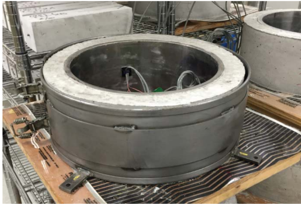
Restrained shrinkage crack ring test setup
