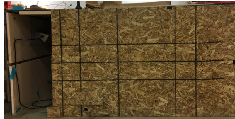
Insulated chamber with infrared heaters
