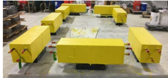
Epoxy painted surfaces
