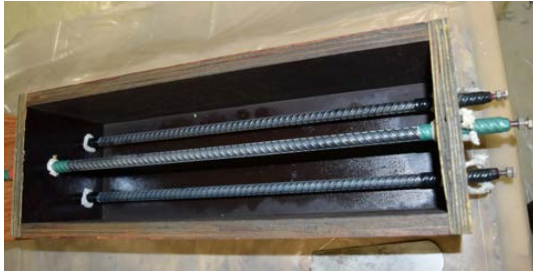
Mold with rebar
