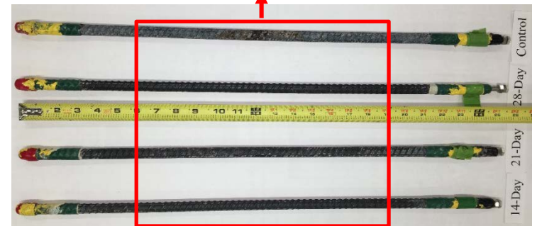
Top rebar of control and treated specimens
