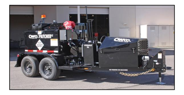
Use only an indirectly-heated melter with sufficient agitation such as the Crafco Patcher II, Crafco Patcher 4, or other approved melter.
